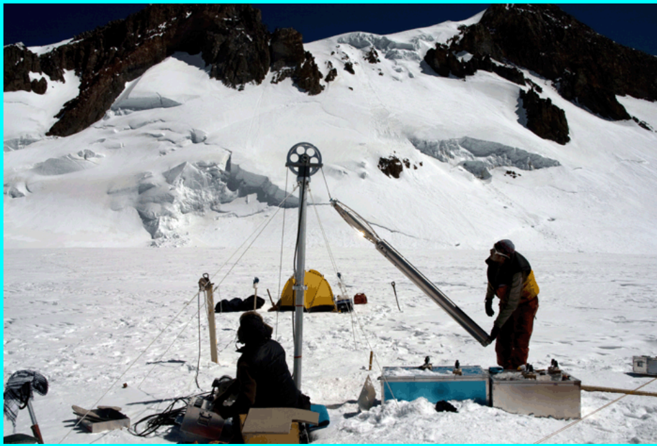
The ice core from the Elbrus plateau was obtained and the structure of ice has been analyzed in 2009-2010
